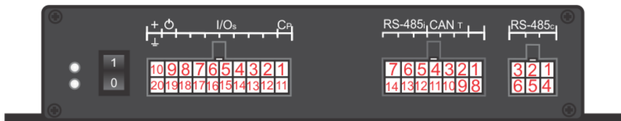
Figure 13: Slave BMS unit connections description.
