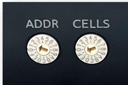
Figure 5: BMS address and cell selection rotary switches.
